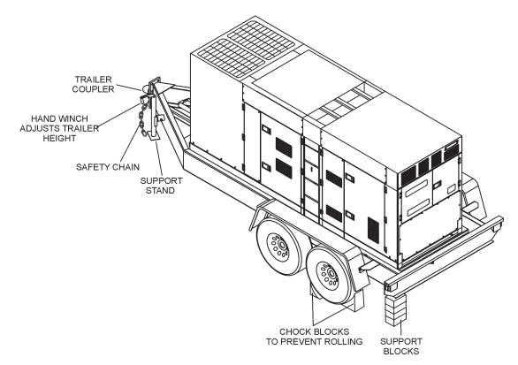
Figure 4. Generator and Trailer
